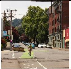
Dashed bicycle lane markings through intersections provide direction for where cyclists should be positioned as they travel through an intersection. They also alert vehicle drivers that cyclists may be travelling in these lanes.
