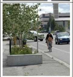
**Bicycle Lanes** are separate travel lanes designed exclusively for bicycles. The lane is defined by white pavement markings and signage.
