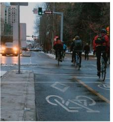
**Protected Bicycle Lanes / Cycle Tracks** are bicycle only facilities that are physically separated from vehicle travel lanes. They can be roadside or on-street, raised or at grade, one- or two-way, and combine the experience of an off-street path with the onstreet infrastructure of a conventional bicvcle lane.
